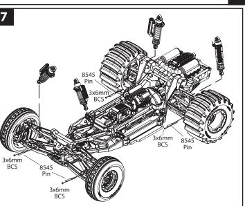
Reattach the lower shock mounts of all four shocks to the suspension arms.
