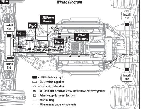
Install the underbody lights on the mounts in the order shown in the wiring diagram using the included 2.5x10mm cap screws. Reinstall the upper pins and screws removed in Step 1 for all four shocks.
